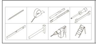
drills hammer drill, ladder/scaffolding, screwdriver, hammer measure tape, pencil/marker, spirit level, ring/flat wrenches, Allen keys, anchors.
