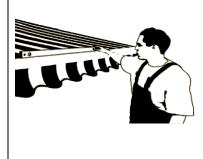
18) After changing the tilt angle, remember to modify the position of the roller tube support.
