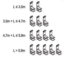
It is recommended to mount the outer wall brackets at a distance of 20 to 45 cm from the ends of the awning, and place the remaining brackets at equal intervals.
