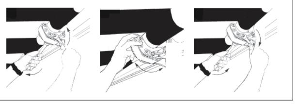
The half-rings of the roller tube support should be adjusted in accordance with the pictorial manual (below).
