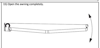
16) To change the tilt angle of the awning use an Allen wrench to loosen (increase the tilt angle) or tighten (decrease the tilt angle) adjusting screws of the arm brackets, then tighten the screw.
